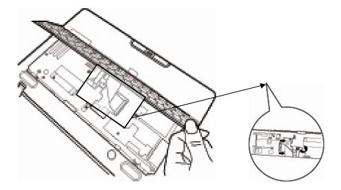
Figure 4-14 Disconnecting the keyboard flexible and LED cable
